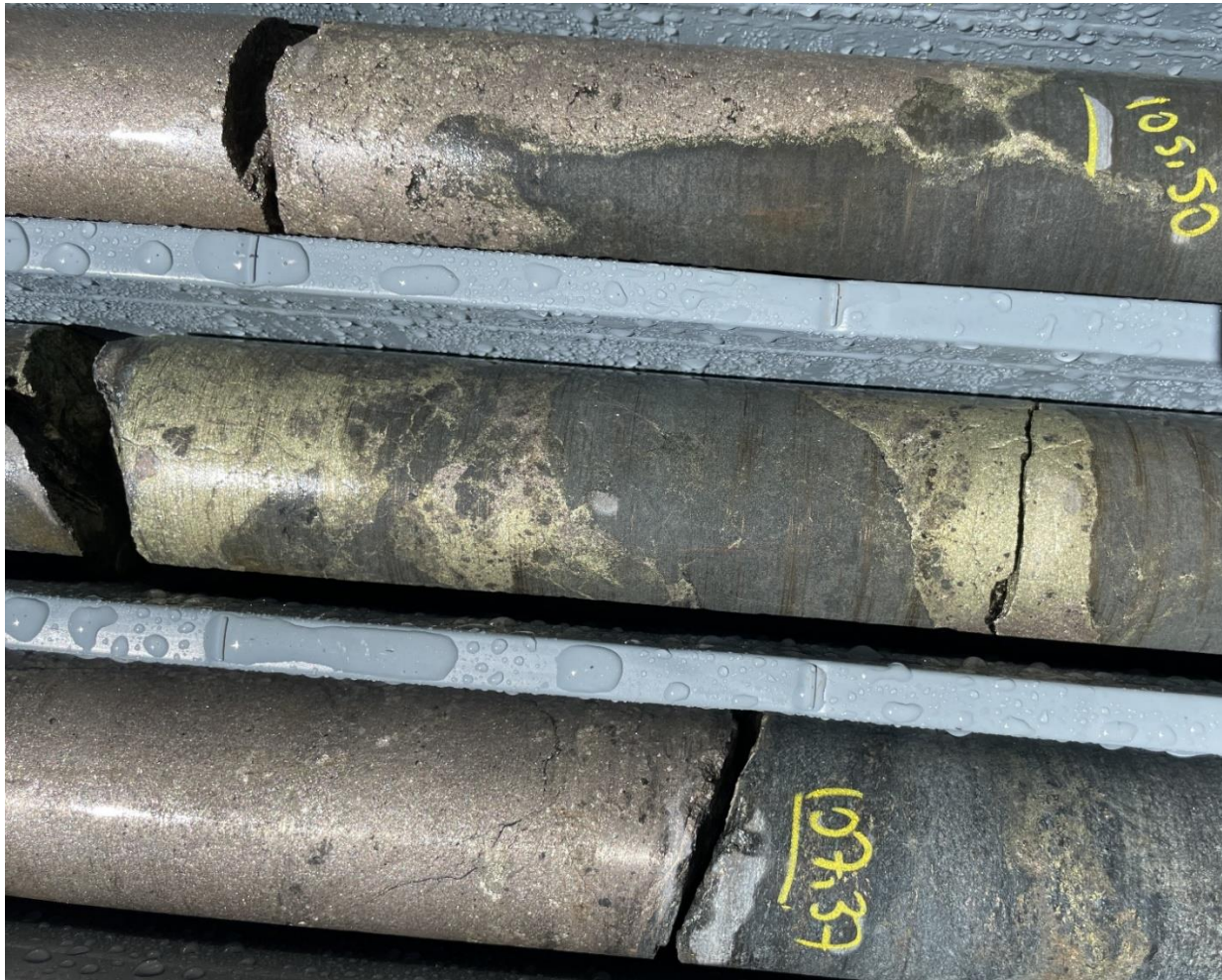
Figure 3: 22B2DD017 (105.08-107.37m interval – NQ core 47.6mm diameter). Further detail of this strongly mineralised dolerite, seen in Figure 2 above, with bands of fine-grained massive pyrrhotite and coarser pentlandite, along with a zone of chalcopyrite-pyrrhotite-pentlandite. Within a 38.94m zone of sulphide mineralisation. 1
