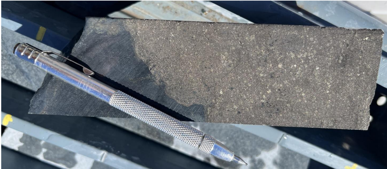
Figure 6: 22B2DD013 (109.46-109.67 interval – cut NQ half-core 47.6mm diameter). Strongly mineralised dolerite with fine-grained massive pyrrhotite mineralisation with coarse minerals of chalcopyrite, within an 18.54m zone of sulphide mineralisation. 1
